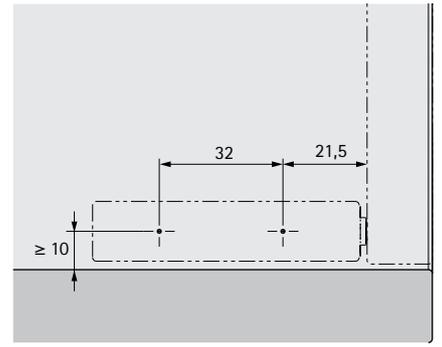
Drilling jig for Push to open
