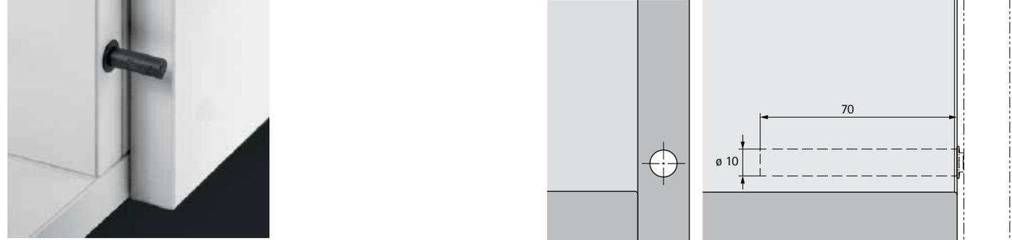
Drilling pattern for the attachment housing for overlay or inset door with Push to open Pin
