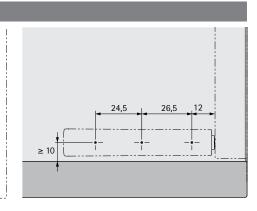
Drilling pattern for short version, overlay door
