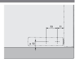
Drilling pattern for long version, overlay door or inset door
